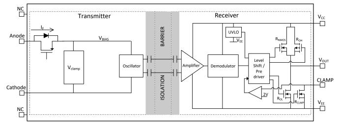
图 8-2. Functional Block Diagram for UCC23514M (Miller clamp)
