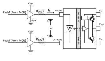
$$R_{EXT} = \frac{V_{SUP} - V_F}{I_F} - (R_{OH\_buf} + R_{OL\_buf})$$
