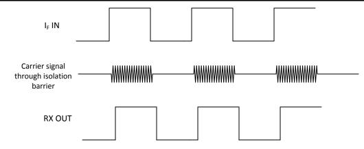
图 8-5. On-Off Keying (OOK) Based Modulation Scheme
