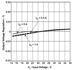
Figure 12. Output Voltage Regulation % vs. Input Voltage
