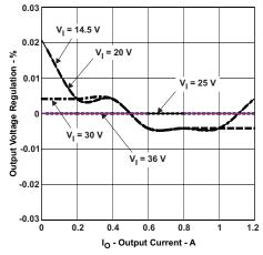
Figure 11. Output Voltage Regulation % vs. Output Current
