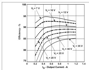
Figure 19. Efficiency vs. Output Current
