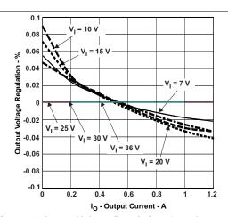
Figure 20. Output Voltage Regulation % vs. Output Current
