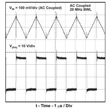
Figure 13. Input Voltage Ripple and PH Node,  $I_0 = 1$  A
