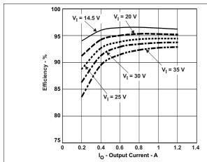
Figure 10. Efficiency vs. Output Current
