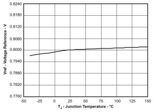
Figure 6-4. Voltage Reference vs Junction Temperature
