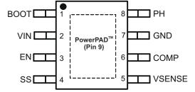
Figure 5-1. 8-Pin SOIC D Package (Top View)
