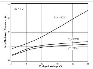
Figure 6-2. Shutdown Quiescent Current vs Input Voltage
