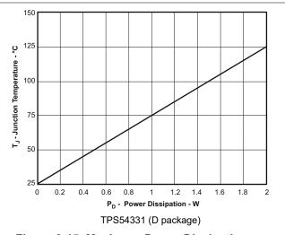
Figure 8-15. Maximum Power Dissipation vs Junction Temperature
