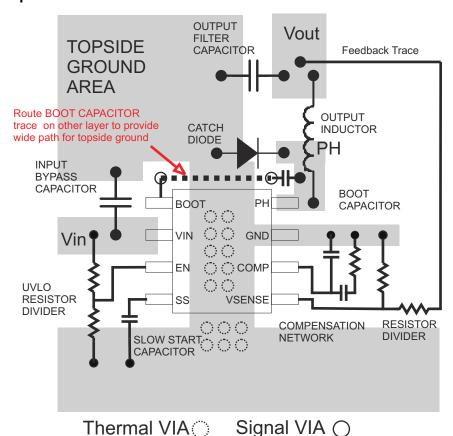
Figure 10-1. TPS54331 Device D Board Layout
