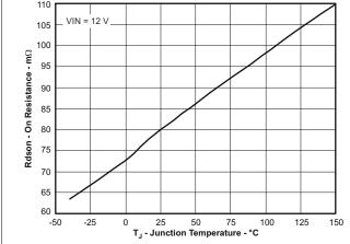
Figure 6-1. ON Resistance vs Junction Temperature
