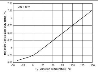
Figure 6-6. Minimum Controllable Duty Ratio vs Junction Temperature
