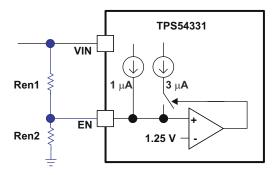
Figure 7-1. Adjustable Input Undervoltage Lockout
