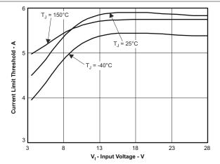
Figure 6-8. Current-Limit Threshold vs Input Voltage
