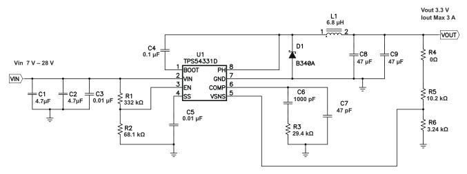
Figure 8-1. Typical Application Schematic
