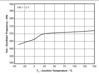
Figure 6-3. Switching Frequency vs Junction Temperature
