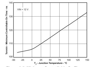
Figure 6-5. Minimum Controllable On Time vs Junction Temperature
